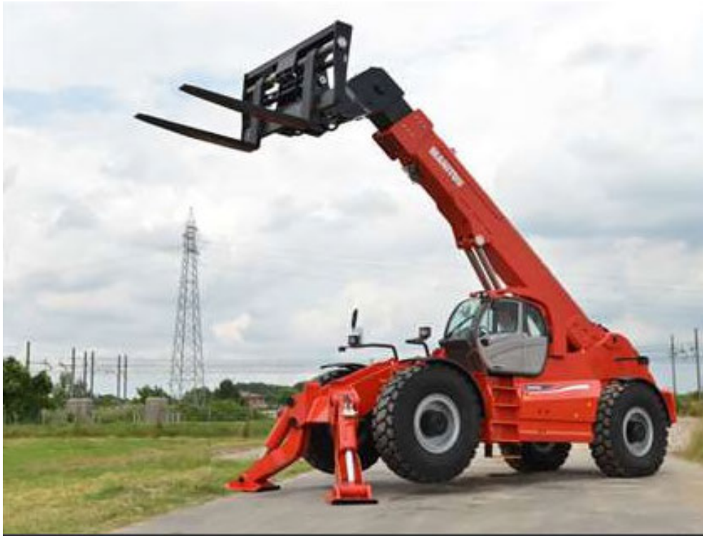
Figure 1.5 – Typical telehandler for loading/unloading deliveries at the erection point.
