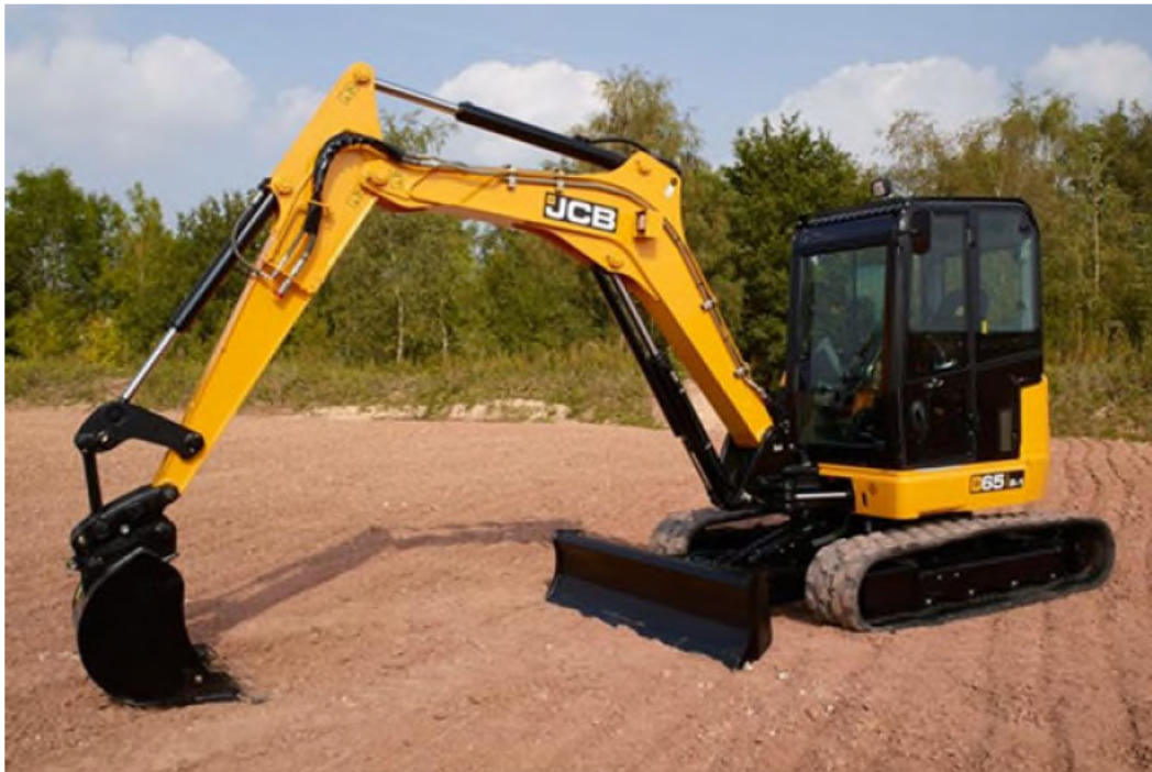
Figure 1.3 – Typical 6T excavator for ground works and levelling.
