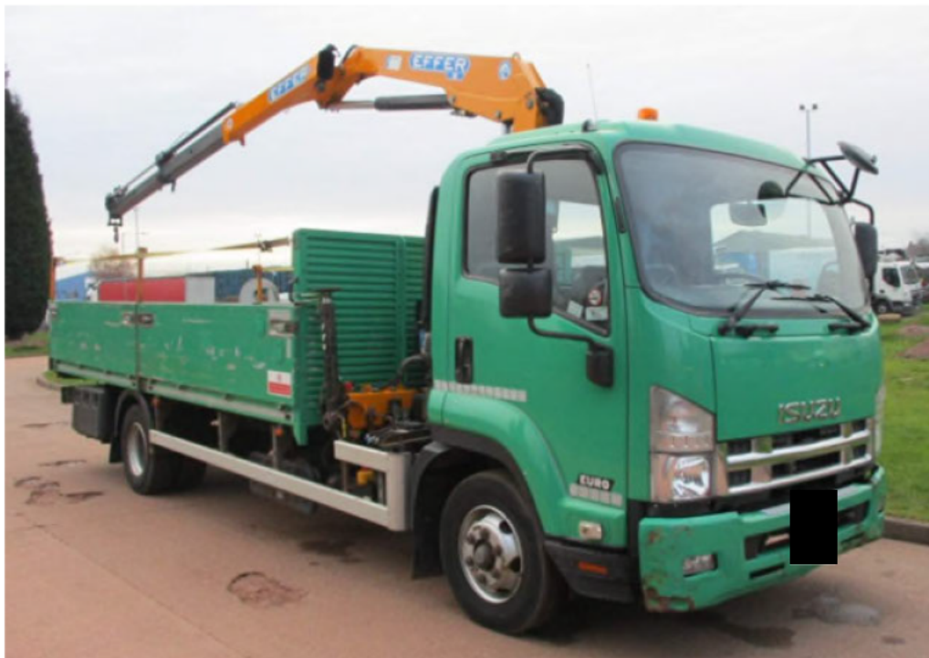
Figure 1.4 – Typical crane lorry for delivery of scaffolding & temporary bridge.
